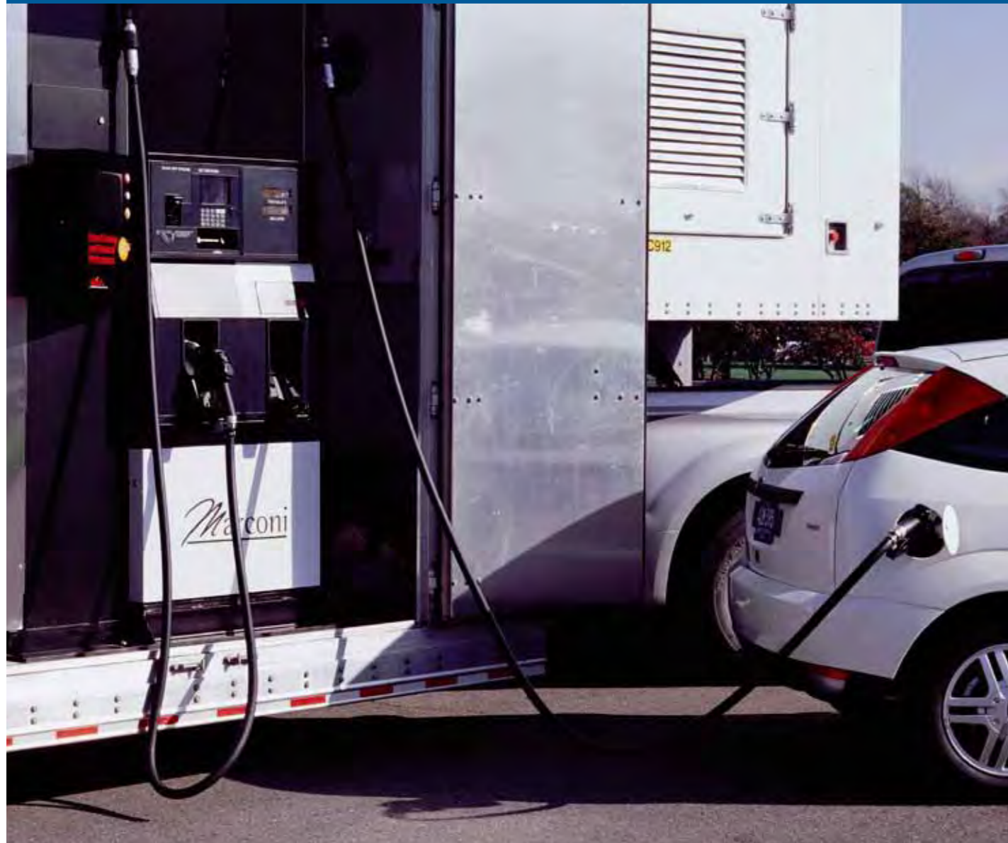
Demonstration of co-fuelling of diesel and urea for a Diesel Ford Focus vehicle, designed to meet Californian ULEV II emission standards
