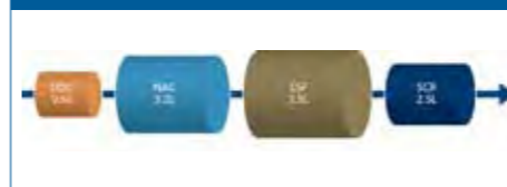
Figure 1: Diagram of catalyst configuration as equipped on the test vehicle.
