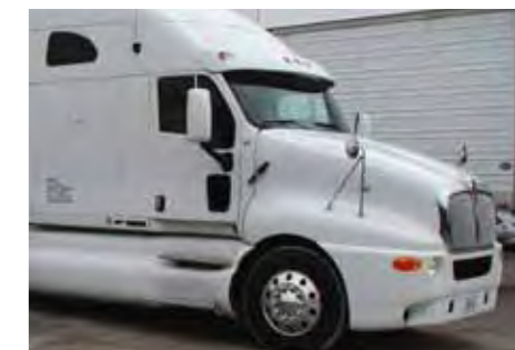
Figure 2: This SCRT ® -fitted truck drove 125,000 miles with no loss of NO x conversion efficiency
